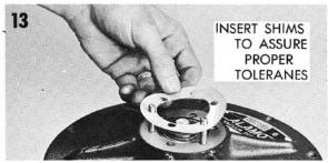
PROPERLY SET) on the rotor assembly and check to see that the end plate is resting squarely on the rotor. Gently tap the bearing onto the shaft and into the end plate to get bearing started. Using the longer 5/16" bolt with washer, pull the bearing into place. Remove longer bolt and replace with grade 5 bolt, lockwasher and positioning washer, and tighten to 200 in-lbs. A thread locking sealant is also recommended to prevent the bolt from backing out.
