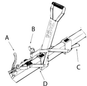
The lever mechanism of the VINK calf puller with alternate traction is equipped with 2 hooks which will be drawn backwards one by one when pulling the handle backwards. The distance between the two hooks when pulling is approximate 7 cm (2.75 in). The distance between the knots in the ropes must be the same to ensure equal traction on both legs of the calf.
