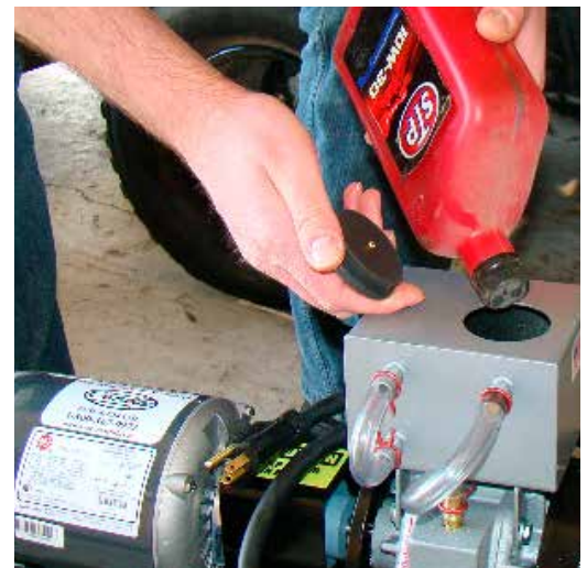
Adding oil to the oil reservoir.
