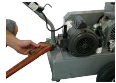
As the oil runs through the vacuum pump it is discharged into the exhaust chamber in the back portion of the tank. The oil will settle to the bottom and the air will be exhausted thru the 3/4" pipe elbow toward the top of the chamber. If the pump is run for a long period of time in the same position, a small amount
