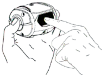
Fig. 5 Main slide removal
