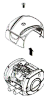
Fig. 6 Dismantling the reversing mechanism block
