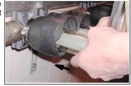
The milking shells must be inserted horizontally into the rinsing receptacle.
