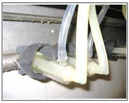
To remove the milking shell from the CIP unit, lift up the back slightly and then pull out.
