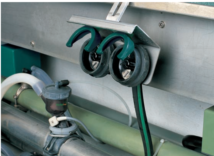
The milking unit holders are sized precisely for the TopFlow Z and TopFlow S, ensuring reliable cleaning of the teat cups during the CIP process. The holders integrate easily into any milking parlor for trouble-free operation.
